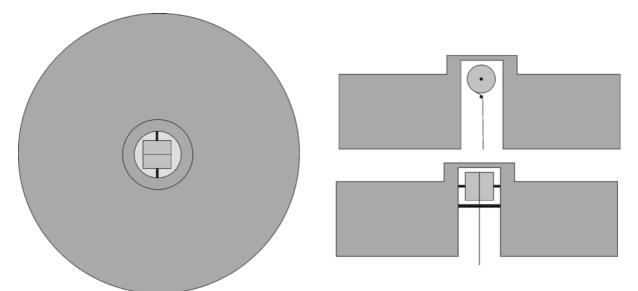
**Figure 5.8** A hollow buoy with a raised head and guide wheel. The raised head increases the distance between the drum and the water surface. This is to decrease the chances of wetting and biofouling of the moving parts. Clockwise from left: view of the buoy from above, view from the side and view from the front.
