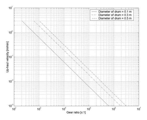
**Figure 7.5** *The variation of the gear ratio on up-haul velocity at different drum diameters. This is with a motor working at 2000 rpm.*
