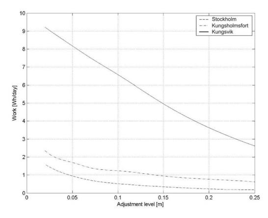
**Figure 7.2** The graph shows how the power need of the regulation system for the buoy varies depending on the predetermined limit of adjustment for the three locations; Stockholm, Kungsholmsfort and Kungsvik. The work per day is the average work derived from the total work over one calendar year.
