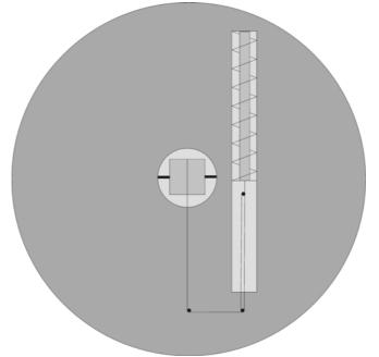
**Figure 5.2** *A hollow buoy with horizontal spring and pulley-tack system. The darker tube inside of the spring is the dampener. (Top view).*
