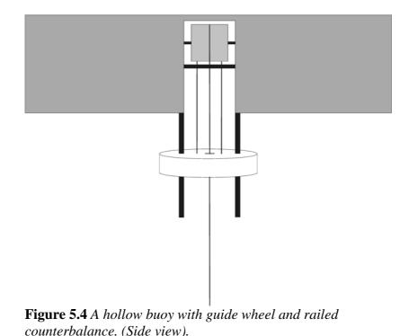
The downsides are increased weight, a more complex buoy design and the possibility of more biological build-up, which in the long term may hinder the weight to travel smoothly. Another problem could stem from the weight being lifted at a skew angle causing it to jam on the guide pole. Having the weight fitted with rollers would counteract this dilemma.
