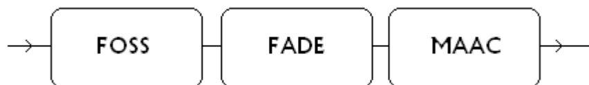
Figure 4: The flow of water through the filters in a full scale application. With enough filter volume, the water does not need to be re-circulated.
