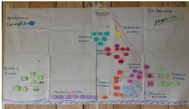
Figure 1 A sketch used to plan the placement of the communal taps in San Salvador. Each colour represents a group of houses that will use one tap and the orange dots represent a communal tap.
