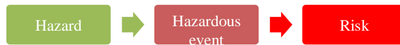
Figure 3 The three main steps in risk assessment. Identify hazards, the hazardous events and then evaluate how big the risk is based on the likelihood that the hazardous event occurs and the severity of the damage it can cause.
