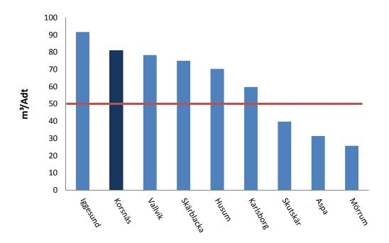
Figure 14. Process water consumption per air dry ton (Adt) in Swedish ECF kraft pulp mills 2010 (Skogsindustrierna, 2011). The red line represents the highest value of the BAT standard interval.
