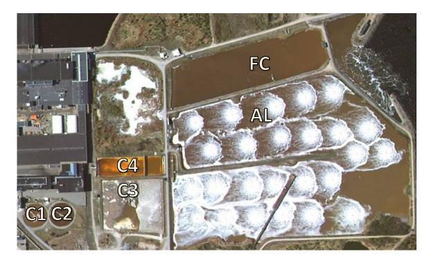
Figure 15. An overview of the external wastewater treatment at Korsnäs. The wastewater treatment includes clarifier 1, 2, 3 and 4 (C1, C2, C3 and C4), the aerated lagoon (AL) and the final clarifier (FC) (© Lantmäteriet, permission I2012/0021, 2012).
