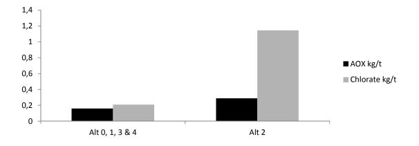
Figure 30. AOX and chlorate emissions from Korsnäs for alternatives of wastewater treatment, alternative 2 being MBR on BLP.
