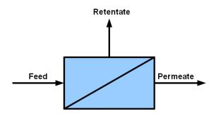
Figure 7. Feed entering a filtration unit, resulting in retentate and permeate.
