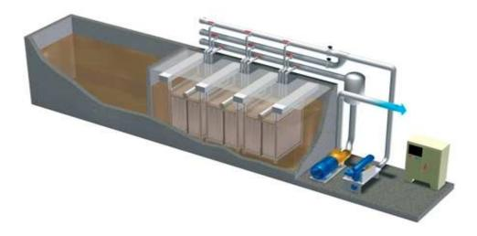
Figure 4. An overview of a submerged MBR equipped with ZeeWeed<sup>®</sup> membranes (GE Water & Process Technologies, 2012).
