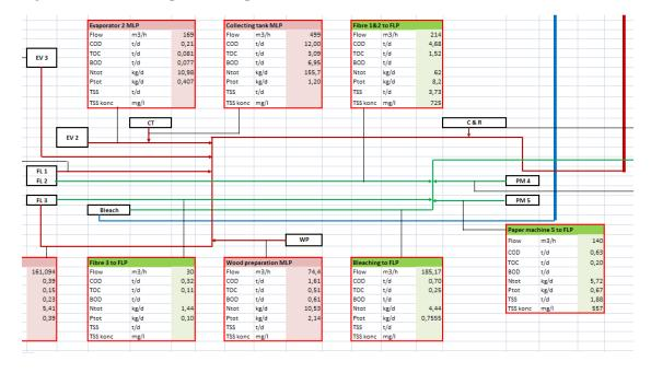
Figure 24. Screen dump of excel spread sheet used for emission calculations.
