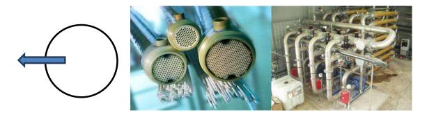
Figure 12. Left to right: Inside to outside permeate flow of MT membranes, Wehrle MT membranes and Wehrle MT membrane modules at site.
