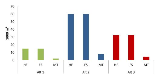
Figure 27. Required membrane area for alternative 1, 2 and 3, using HF, FS or MT membranes.
