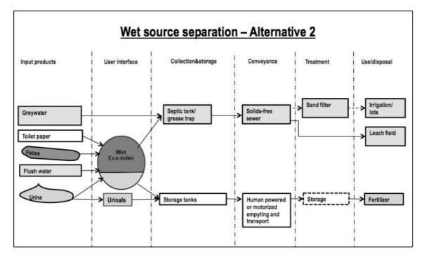
Figure 27. Schematic overview of functional groups for wastewater system sand filters/leach fields.
