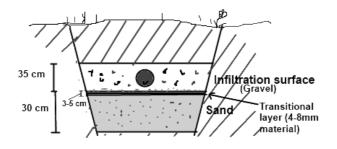
Figure 33. Layer depths for reinforced leach fields, reasonable total depth of about 1 m (Authors's figure inspired by Naturvårdsverket (2003)).
