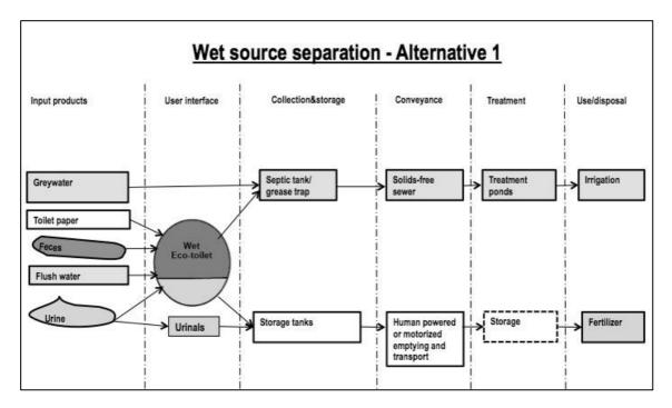
Figure 26. Schematic overview of functional groups for wastewater system with treatment ponds.
