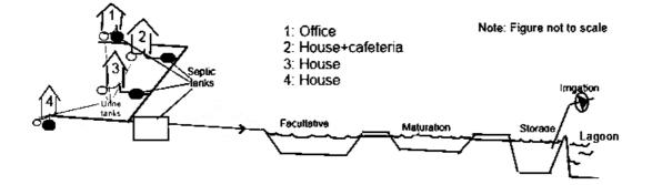
Figure 28. Schematic overview of suggested wastewater management, Alternative 1.
