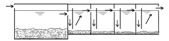
Figure 20. Baffled reactor (Author's figure, inspired by Sasse (1998)).
