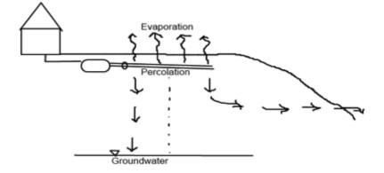
Figure 23 Fate of water discharged to onsite wastewater treatment systems (inspired by EPA, 2010).
