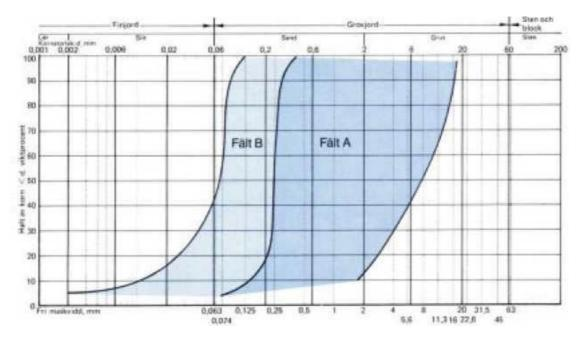
Figure 24. Suitable soils for leach fields, Zone A ("Fält A") in dark blue and Zone B ("Fält B") in lighter blue (Source: Naturvårdsverket, 2003, with permission).
