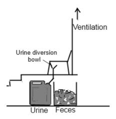
Figure 17. Eco-toilet. Urine is collected from the front of the toilet while feces are collected from the back.
