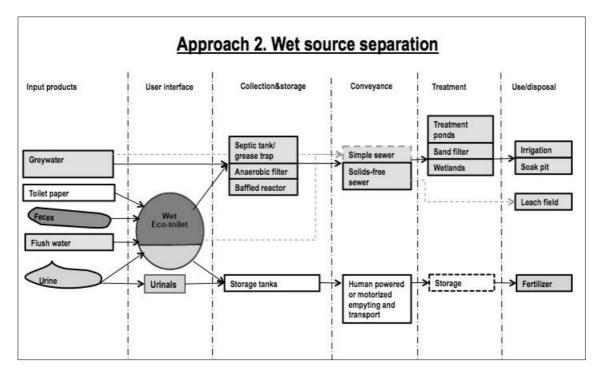
*Figure 15. Schematic sketch of the wet source separation approach (Author's figure inspired by Tilley et al. (2008)).*
