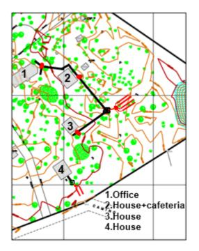
Figure 32. Present sewer (in black) and possible leach field placement (in red) combined for three buildings (Source: Modified from Ceasip (2008)).
