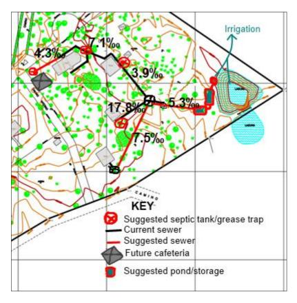
Figure 29. Approximate sketch of current sewer, suggested sewer, suggested septic tank locations and slopes at Ceasip (modified from Ceasip, 2008).
