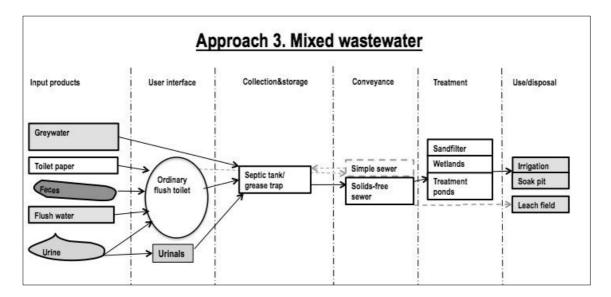
Figure 16. Schematic sketch of the mixed wastewater approach (Author's figure inspired by Tilley et al. (2008)).
