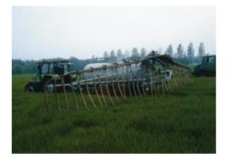
Figure 22. Tankwagon with trailing hoses (Source: Johansson et al. (not dated), with permission).
