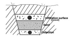
Figure 21. Cross-section of horizontal sand filter (Author's figure inspired from Naturvårdsverket, 2003).
