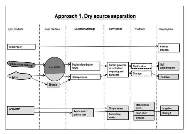
Figure 14. Schematic sketch of the dry source separation approach (Author's figure inspired by Tilley et al. (2008)).
