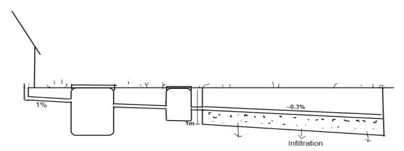
Figure 31. Schematic overview of wastewater management, Alternative 2.
