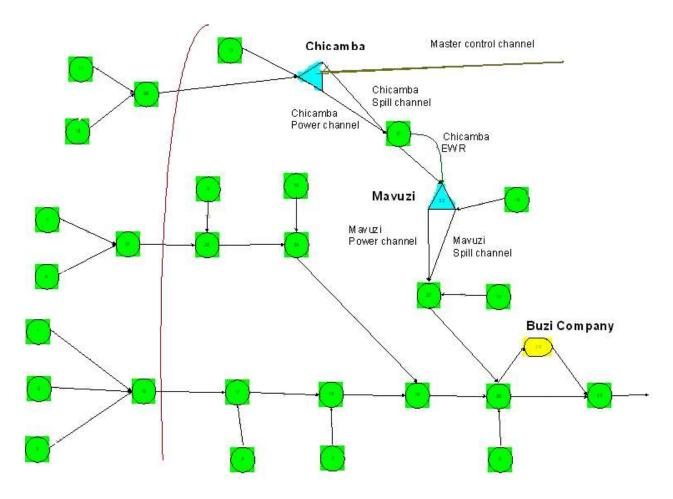
**Figure 5** The Buzi River basin with the analyzed large-scale water consumers, illustrated in the WRYM- IMS. The green dots represent the nodes and the black lines represent flows with directions. The two blue triangles represent the reservoirs of the power plants and the yellow dot represents the irrigation field. The red line illustrates the border between Mozambique and Zimbabwe (illustration by author, recreated version).
