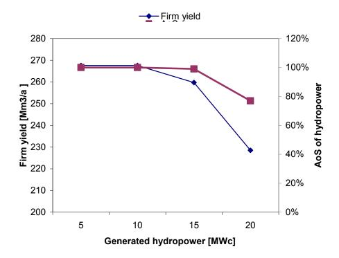
**Figure 12** *Firm yield (at the Chicamba dam) and assurance of supplied hydro power (at the Mavuzi dam) with increasing levels of hydropower generation at the Mavuzi dam.*
