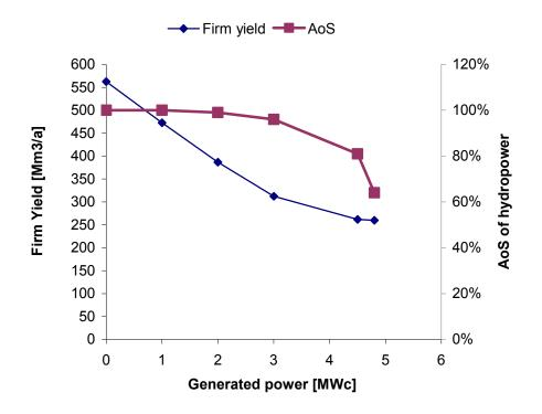
**Figure 11** *Firm yield and assurance of supply of hydropower with increasing demands of generated hydropower, at the Chicamba dam.*
