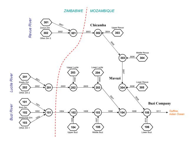
Figure 19 The Pitman flow schematic network of the Buzi River basin (Sweco, 2010)
