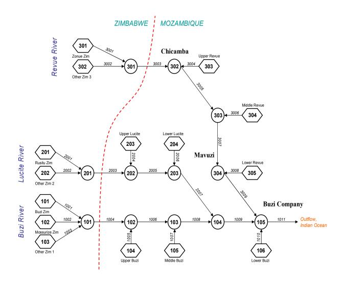
**Figure 6** A flow schematic network diagram for the Buzi River basin, including the water consumers: Chicamba dam (Upper Revue sub-catchment), Mavuzi dam (Middle Revue sub-catchment) and the Buzi irrigation system (Lower Buzi sub-catchment). The hexagonal figures represent the sub-catchments and the nodes represent measurement stations. The red line illustrates the border between Mozambique and Zimbabwe (modified from Sweco, 2010).
