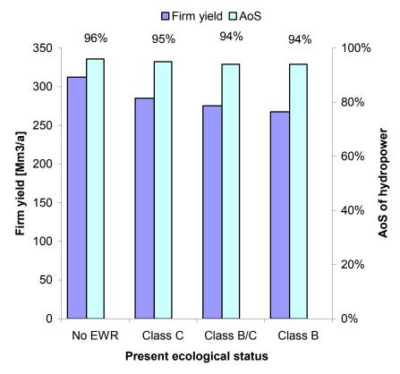
**Figure 13** *Firm yield and assurance of supplied hydropower with increasing PES, at the Chicamba dam*
