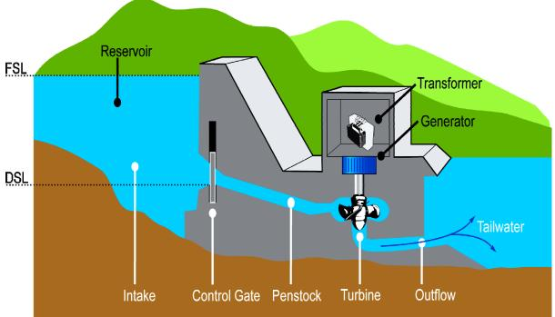
**Figure 2** The typical hydropower plant with its various technical characteristics (author's illustration).
