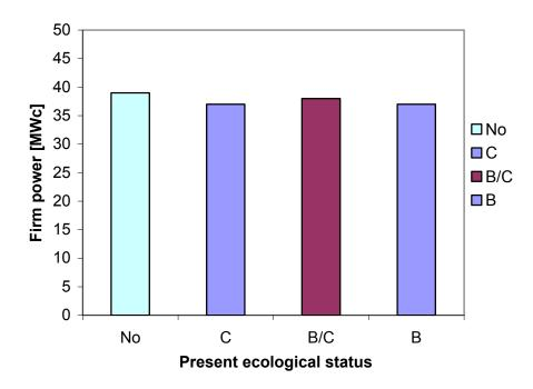
Figure 15 Firm power at the Mavuzi dam with increasing PES of the Chicamba catchment
