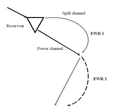
**Figure 16** Alternative locations of an EWR release at the Mavuzi dam. Location number one (grey line) represents the spill channel of the power plant. Location number two, released through the power channel, is located downstream of the power plant.
