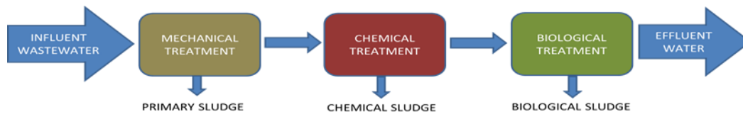
Figure 1 The process of wastewater treatment including mechanical, chemical and biological treatment. Formed sludge from each step is past to sludge treatment, usually an anaerobic digestion process.
