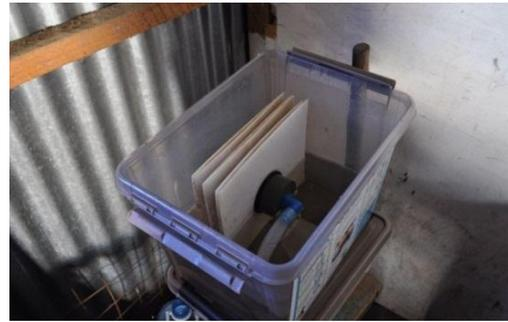
**Figure 26** Filter unit using borehole water in Oloosuyian.
