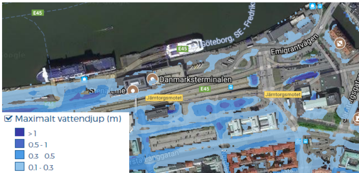
Figure 5: Simulation result of a rain by return period of 100 years for Masthuggskajen (Göteborgs Stad, 2015a).
