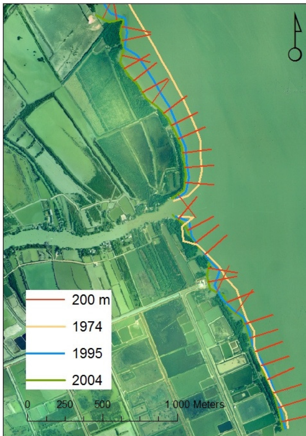
Figure 5.5. Visualisation of the movement and former location of the coastline in 1974 and 1995. Aerial photo from 2004.
