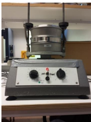
Figure 4. Electrical sieving machine used for shaking sieves to distribute particles with different sizes
