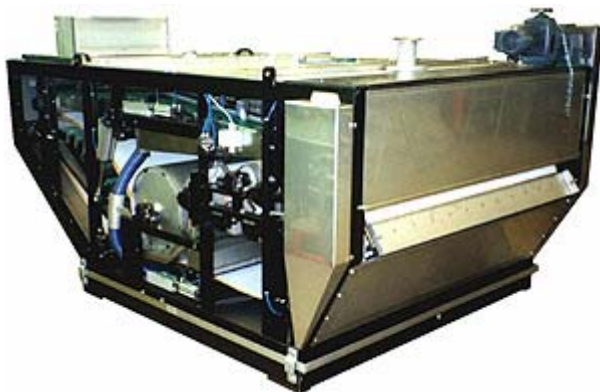
Figure 18. Finish dewatering filter press at Shaha WWTP (Slamex, 2007).
