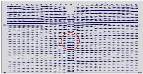
**Figure 25** Primaries-plus-multiples stacked section of zero-offset VSP integrated between crossline 1107 and inline 1172 (the CDP corresponding to borehole 202/2007).
