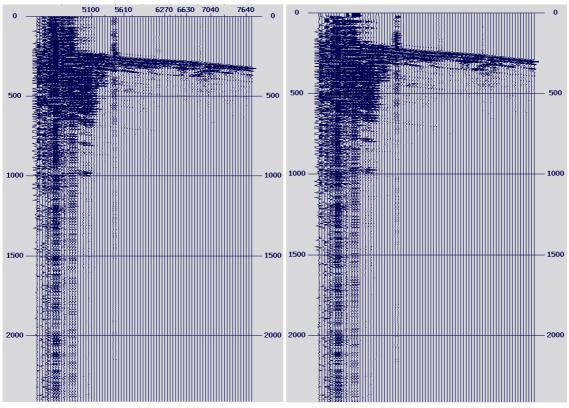
**Figure A7** V component of shot 4010 after synthetic trace interpolation of deleted traces.
