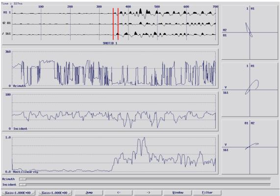
Figure A2 The rotation tool in Claritas used for rotating the azimuth angle.
