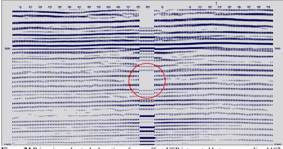
**Figure 24** Primaries-only stacked section of zero-offset VSP integrated between crossline 1107 and inline 1172 (the CDP corresponding to borehole 202/2007).
