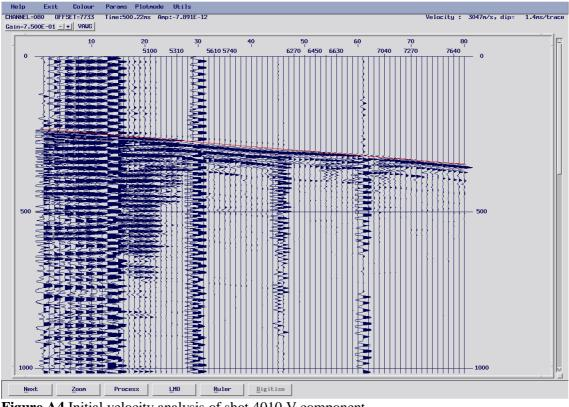
Figure A4 Initial velocity analysis of shot 4010 V component.
