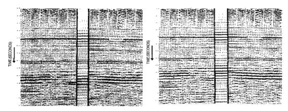
Figure 13 Seismic data correlated with (left) primary zone VSP composite and (right) VSP composite, recorded above the major multiple generating layer (Hamson and Mewhort 1983).
