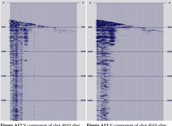
Figure A12 V component of shot 4010 after alignen coherent upgoing energy horizontal.
