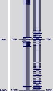
**Figure 23** Correlation between VSP and synthetic trace (with multiples), using velocity model 5.
