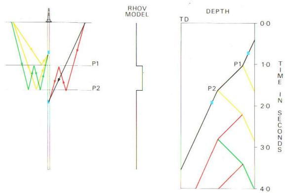
Figure 10 Schematic of ray paths and event pattern for 3-layer model (Kennett et al., 1980).
