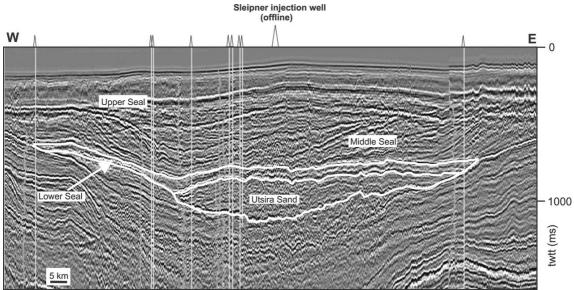
**Figure 5** Regional seismic line through southern part of the Utsira formation (Chadwick et al., 2004).
