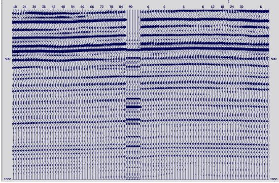
**Figure 30** Primaries-only stacked section of 1042 integrated between crossline 1115 and inline 1196 (the CDP corresponding to midpoint between shot offset and borehole).
