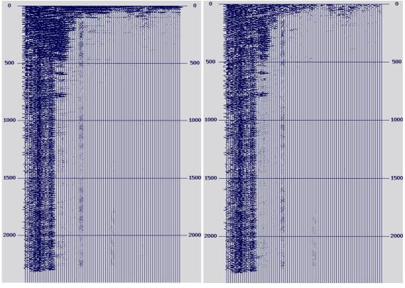
**Figure A10** V component of shot 4010 after alignen coherent downgoing energy horizontal.
