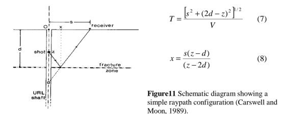
Where V is the velocity of the upper layer, s is the horizontal source offset from the borehole, d is the depth of the layer, x is the offset to the CDP location, z is the depth. In conventional seismic surface surveys, the CDP lies at the midpoint of shot-receiver spread regardless of the depth of the reflector. In the VSP configuration, the CDP migrates horizontally through the subsurface as a function of reflector depth. As the
