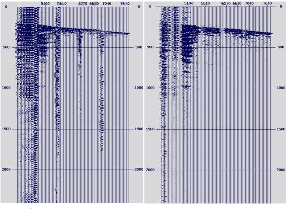
**Figure A5** V component of shot 4010 after bulk static shift and refraction static.
