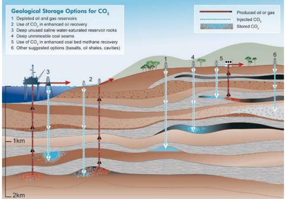
Figure 3 Options for storing CO<sub>2</sub> in deep underground geological formations (IEA, 2004)
