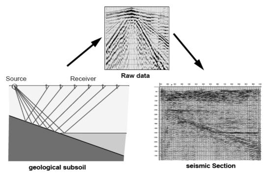
Figure 1 Schematic picture over the seismic methodology (Kruk, 2005).
