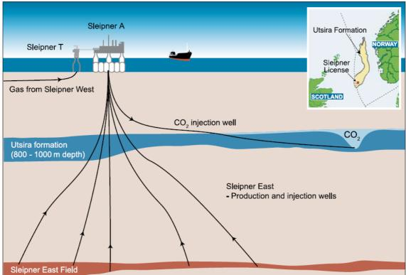
**Figure 4** Simplified diagram of the Sleipner CO<sub>2</sub> Storage Project. Inset: location and extent of the Utsira formation (IPCC, 2005).
