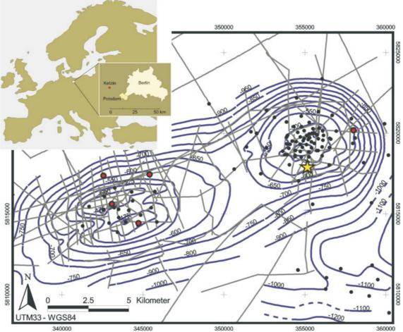
**Figure 8** Index map of the Roskow-Ketzin anticline. Boreholes are shown as dots. Gray lines denote seismic lines of former exploration at Ketzin. The CO<sub>2</sub>SINK injection borehole location is marked with a yellow star. Contour interval of the Heldburg-Gips isolines is 50 m (http://www.co2sink.org, 2008).
