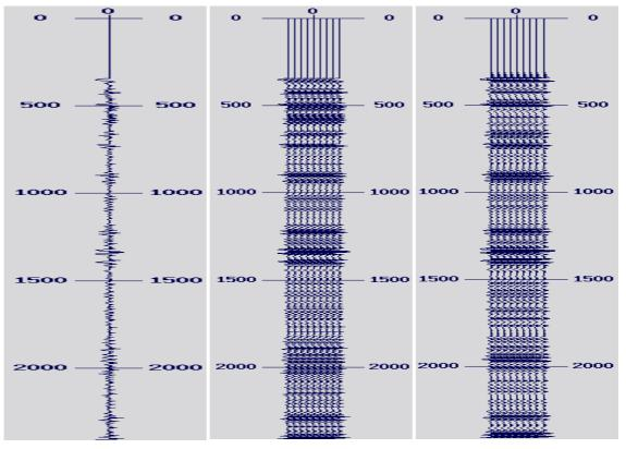
Figure A16 V component of shot 4010 after vertical stacking
