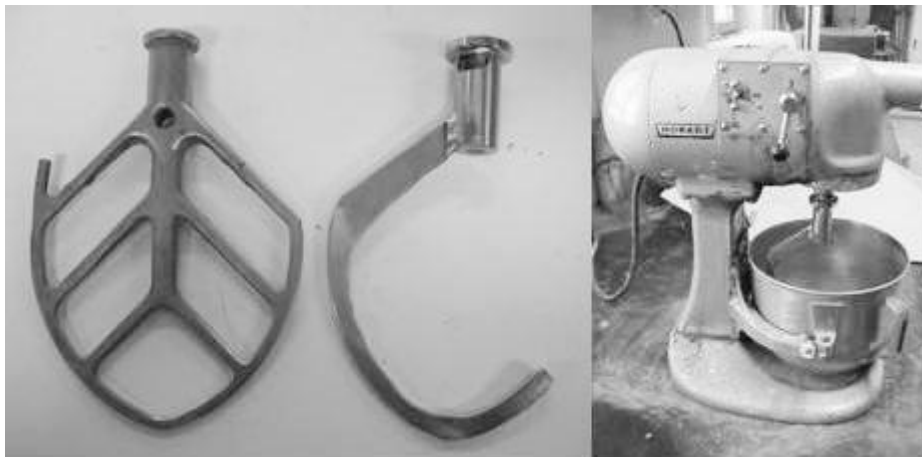
Fig. 6 Photograph of flat whisk (left) normally used for cement, hook shaped whisk (centre) better for mixing clay soils, Hobart mixer (right) used for mixing the soil and the binding agents.
