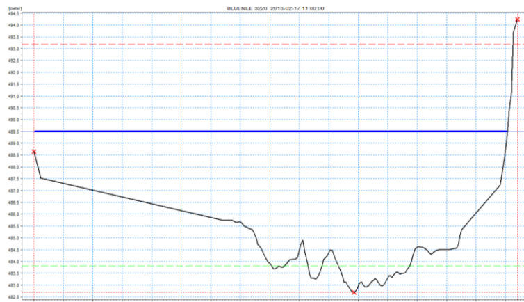
Figure 28 The cross section data for the cross section 6 km downstream of El Deim. The blue line illustrates the current water level, the red dotted line the maximum water level and the green dotted line the lowest water level during an on-going result simulation.
