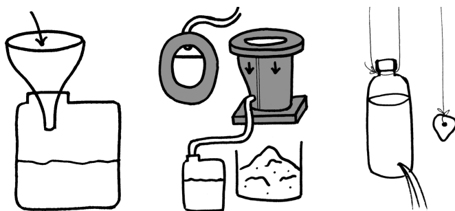
Figure 27 Urine-diverting interfaces, enabling nutrient recovery from urine and reducing problems with odor and flies in the pit: an eco-lily (left) and a urine-diverting pedestal (middle). Simple hand-washing devise (made out of a plastic bottle), hung close to the latrine and accompanied by a bar of soap, to improve hygiene practices (right). Illustration Maria Persson
