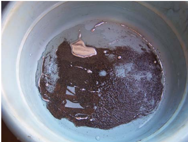
Figure 6.7. Mercury is used for flocculating gold, this can pollute the water and the environment (Photo Lovisa Lagerblad).
