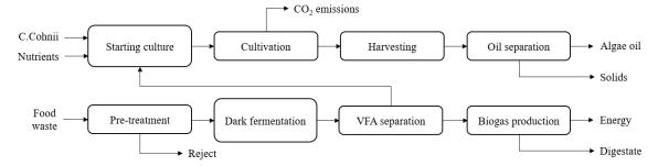
Figure 4: Theoretical DHA production process using VFA from food waste as feedstock to microalgae. Additional energy, water, transports and processing units are required but is excluded in this illustration.
