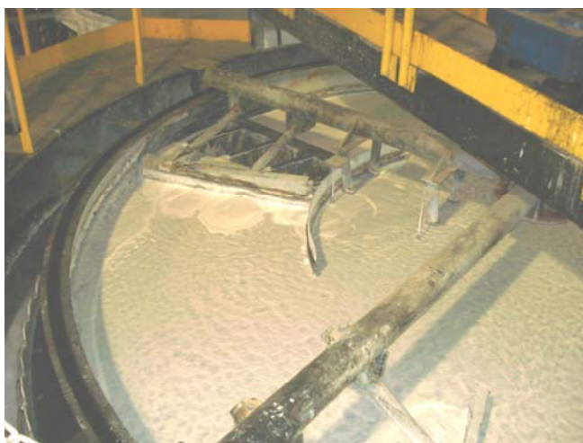
Figure 13. Sludge scrapes at the surface of the flotation tank.
