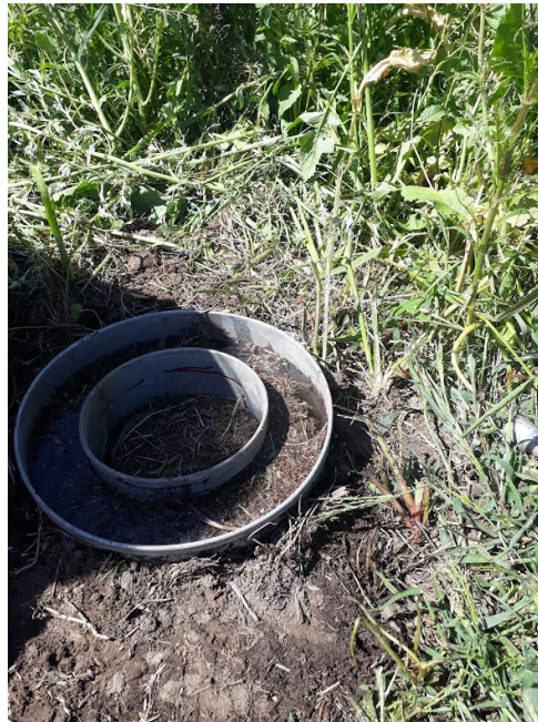
Figure 10: Experimental set-up at “media loma”. In the inner ring the line is marking 4,5 cm, that is the height of the water column at each addition of water. In the photo water had only been added to the outer ring. Soil was added to the borders of the outer ring since water leaked out.
