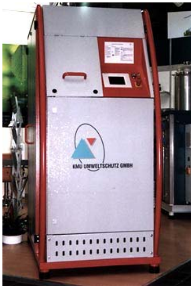
Figure 3: One of Vilokan's evaporators for industrial waste water, Envovap.
