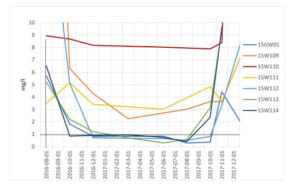
Figure 22. The variation of dissolved oxygen over time for the different groundwater pipes with the time of injection of nutrients marked as a vertical black line. The optimal DO level for reductive dechlorination (USGS, 2006) is marked with a horizontal black line.
