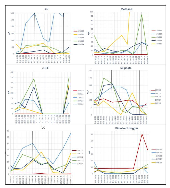
*Figure 26. The levels of methane, sulphate and dissolved oxygen compared to the levels of TCE, cDCE and VC in groundwater pipes 15W110, 15W111, 15W112, 15W113 and 15W114.*
