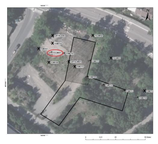
Figure 30. The groundwater pipe 15GW01 is marked in red, and the groundwater pipes not part of the observations are crossed over. The figure is based on WSP:s figure of the area.
