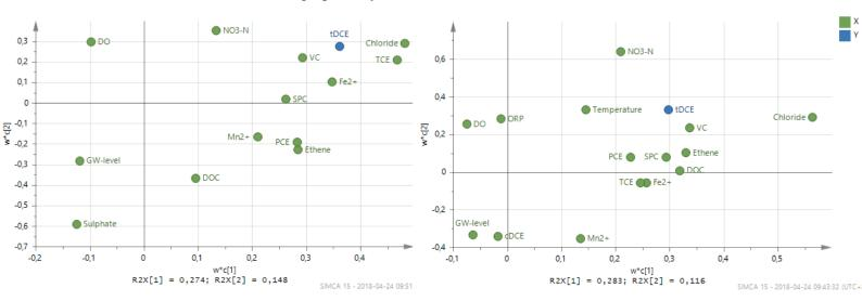
Figure 48. The correlation plot for the non-transformed (above) and log-transformed (below) data with the loadings of the variables.
