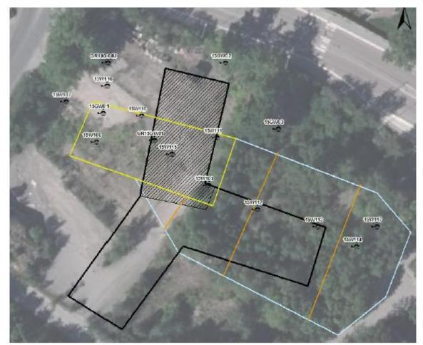
Figure 7. The remediation area (yellow) and plume barriers (orange) to prevent spreading (WSP, 2016b).
