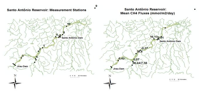
Figure 8 Santo Antônio reservoir: measurement stations and their mean CH<sub>4</sub> fluxes after 30 minutes deployment time.
