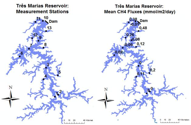
Figure 9 Três Marias reservoir: measurement stations and their mean CH<sub>4</sub> fluxes after 30 minutes deployment time.
