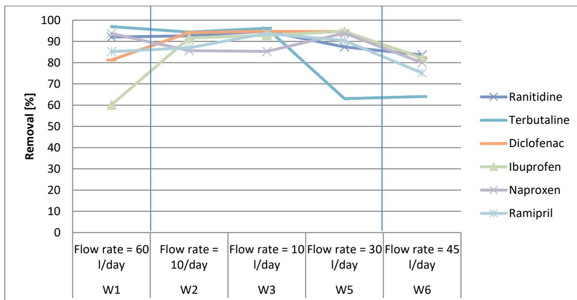
Figure 10. Removal of ranitidine, terbutaline, diclofenac, ibuprofen, naproxen and ramipril achieved by GAC filter A1 during week 1-6, with different loading rates. The substances varied the most during the experiment. The vertical lines (blue) indicate stirring of the upper layers of the filters.
