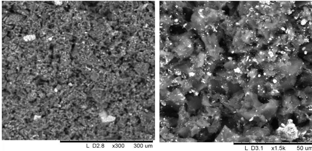
Figure 6. The activated carbon used in the experiment. Left: 300 times magnification. Right: 1,500 times magnification.
