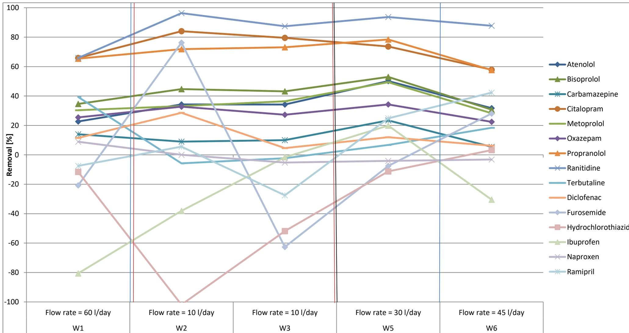
Figure 11. Mean removal of pharmaceuticals with detectable concentrations achieved by bark filters during week 1-6, with different loading rates and bark types. The vertical lines marks the switch from bark <5mm to bark >5 mm(black), floodings (red) and stirring of the filters' upper layers (blue). Note that the last flooding occurred during week four.
