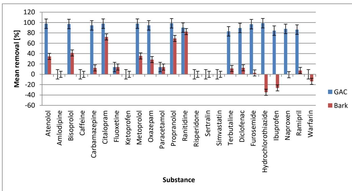
Figure 9. Mean removal of pharmaceuticals for the filters. The error bars show the standard error.
