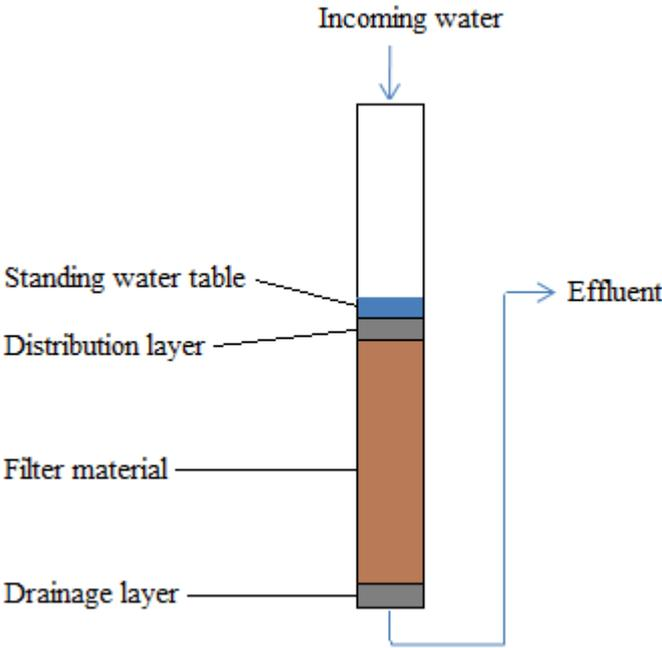
Figure 5. Principle sketch of filters.
