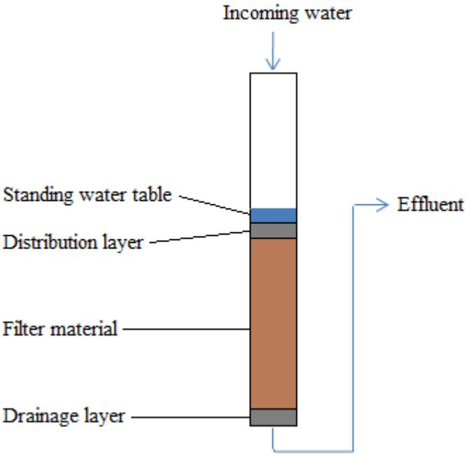
Figure 5. Principle sketch of filters.
