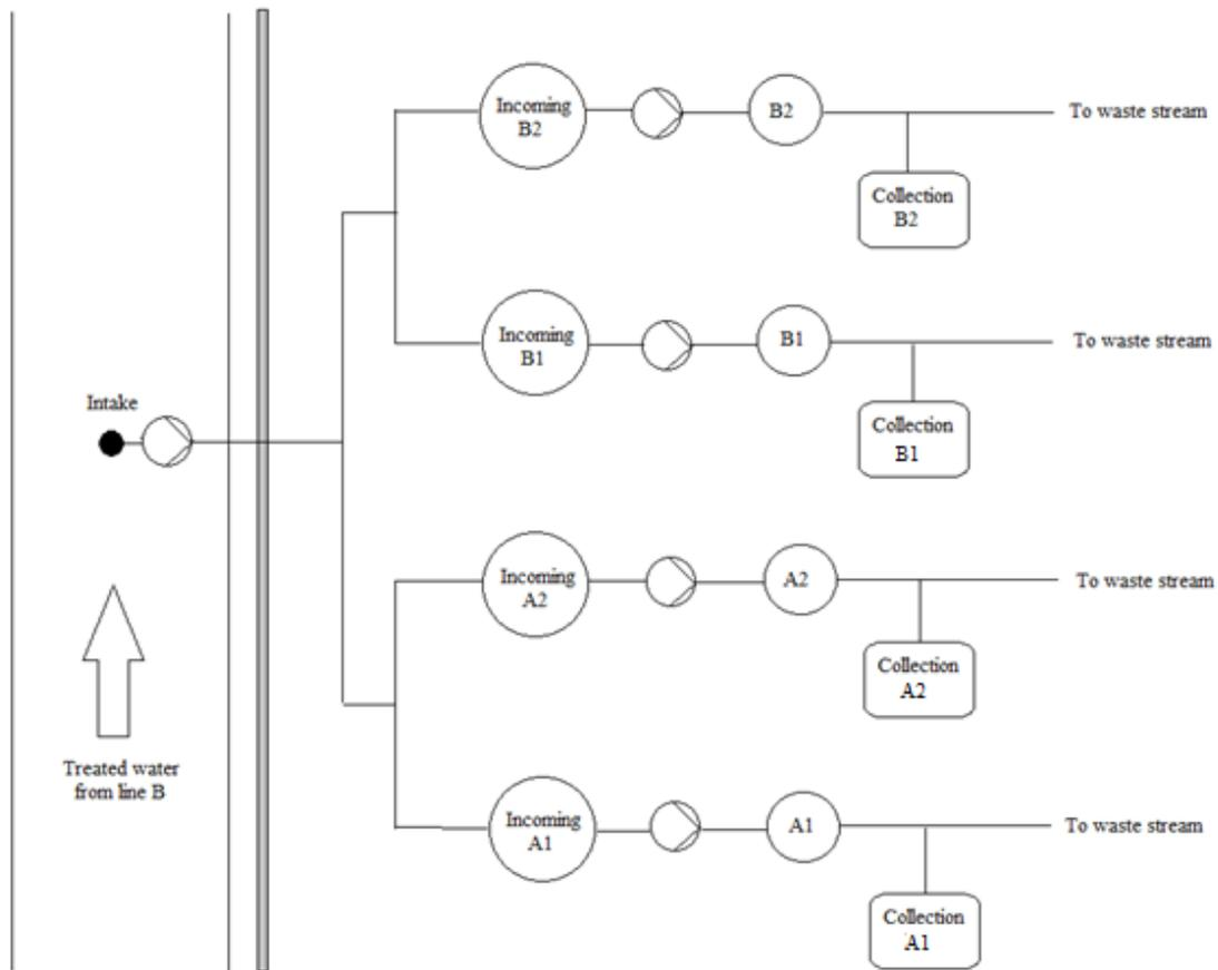
Figure 3. Principle sketch of the experimental set-up which shows the intake of treated wastewater, storage tanks for incoming water, pumps, filters and collection tanks.
