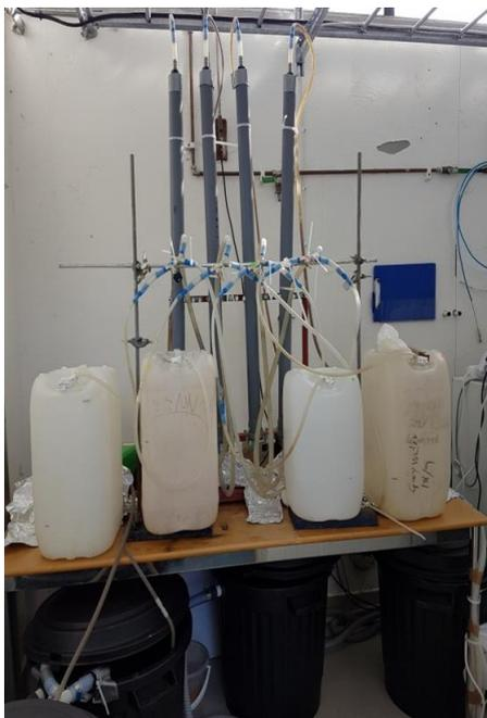
Figure 4. The set-up of the experiment: storage barrels for incoming water (black), collection tanks (white) and filters (grey).
