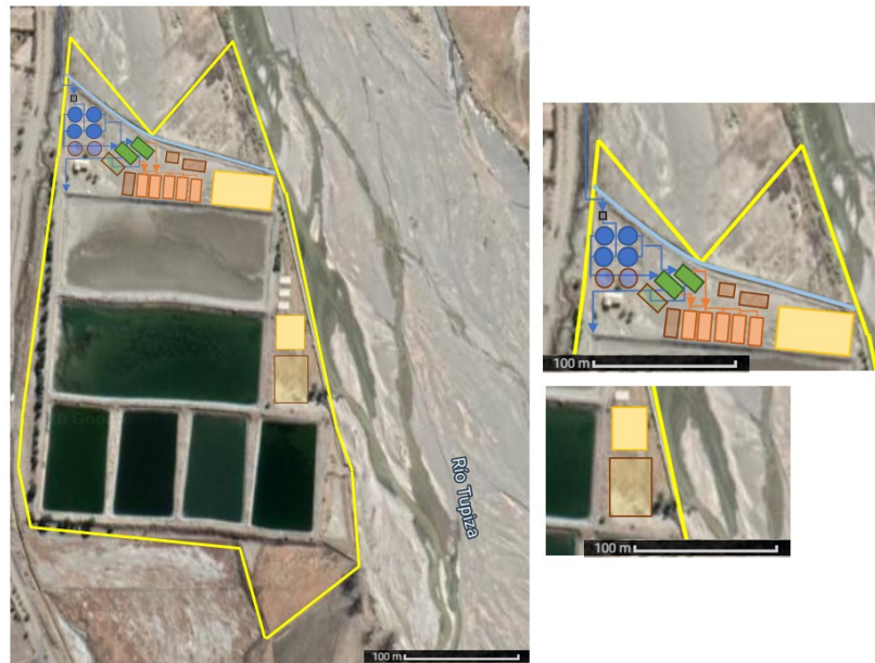
Figure 17: Layout of a potential buildout for option 1. The slightly transparent shapes are added settlers (blue circles), RAC (green box), sludge drying beds (orange boxes) and designated area for hygienization (yellow boxes).
