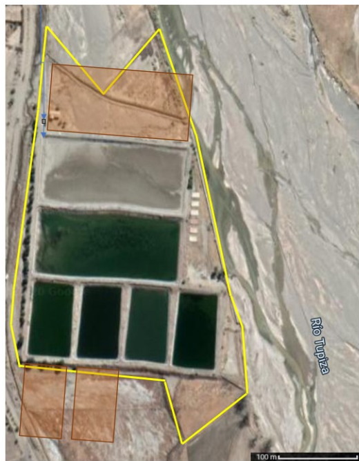
Figure 15: Layout of a potential buildout for option 0. The brown transparent boxes symbolize the buildout in the form of two added maturation ponds and one added facultative pond.
