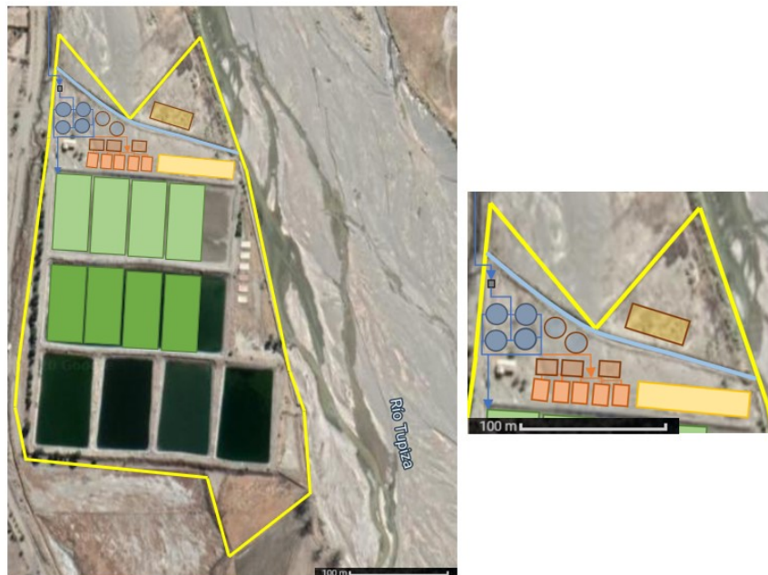
Figure 19: Layout of a potential future buildout for option 2. The slightly transparent shapes are added UASBs (grey circles), sludge drying beds (orange boxes) and designated hygienization area (yellow box). The slightly darker green boxes in the constructed wetland symbolize converted vertical flow wetlands.
