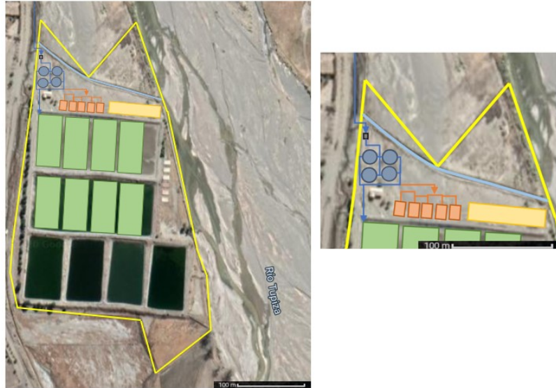
Figure 18: Layout of option 2. The blue circles are the UASBs, the lime green boxes are the constructed wetland and the orange boxes symbolize the sludge drying beds. The yellow box is the designated area for hygienization. The blue and orange arrows show the routes of the wastewater and sludge.
