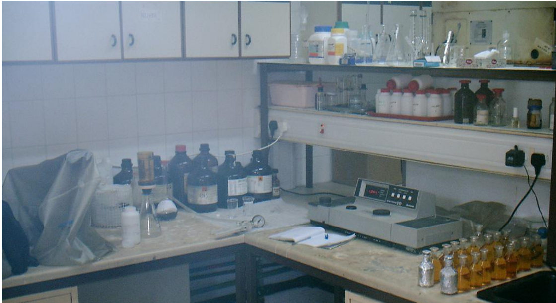
Figure 9 The lab work bench. The filtering equipment with pump is seen to the left and to the right is the spectrophotometer with a collection of sample bottles next to it.
