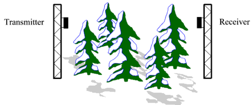
Figure 1. Schematic illustration of a transmission measurement through a forest section.
