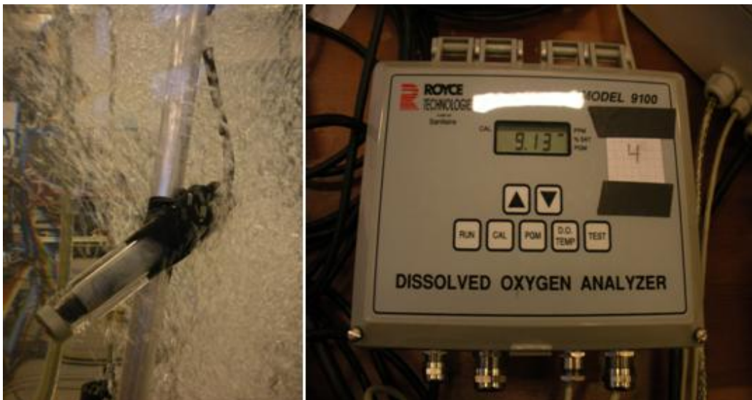
Figure 18 The picture to the left shows a Royce probe which was attached at a steel pole. The picture to the right shows the controller where it was possible to read the dissolved oxygen concentration and the water temperature.
