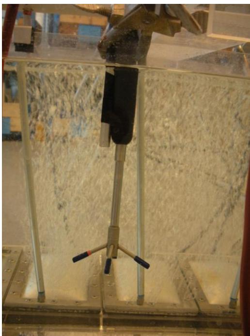
Figure 20 Velocimeter to measure the liquid velocity in the racetrack tank. The instrument has four beams which measures the velocity in three dimensions. The beam with a red line was measuring in the X-direction which in this case was the main velocity.
