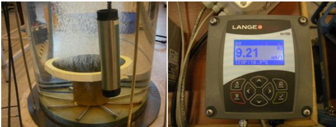
Figure 19 The picture to the left shows the Lange probe. The picture to the right shows the controller where it was possible to read the dissolved oxygen concentration and the water temperature.
