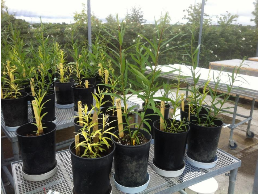
Figure 7 Picture from the experiment in week 7. Plants grown in pyriteash substrates to the left in the picture have clearly been affected in growth compared to the reference plant in the middle (no 18).
