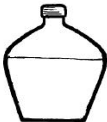
Figure 5 Storing drinking water in narrow mouthed containers prevents from using e.g. ladles or jugs, in other words contaminants are kept from entering the container (with permission from Conant & Fadem 2008).
