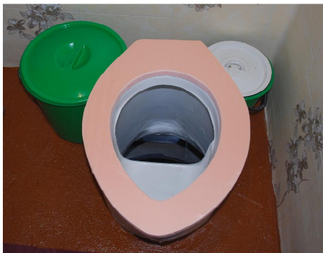
Figure 12 Urine separation toilet with a Styrofoam seat (photo by Katja Larnholt).
