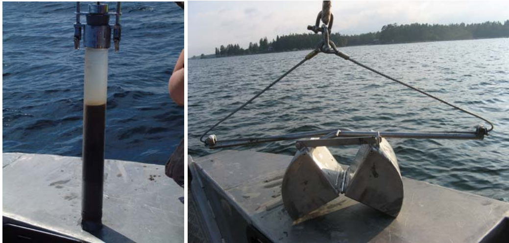
a) b) Figure 8. a) Kayak sediment sampler. b) van Veen grab sampler
