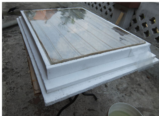
Figure 17 Shows the improved device of the solar water pasteuriser, here on a bamboo frame placed on a table.
