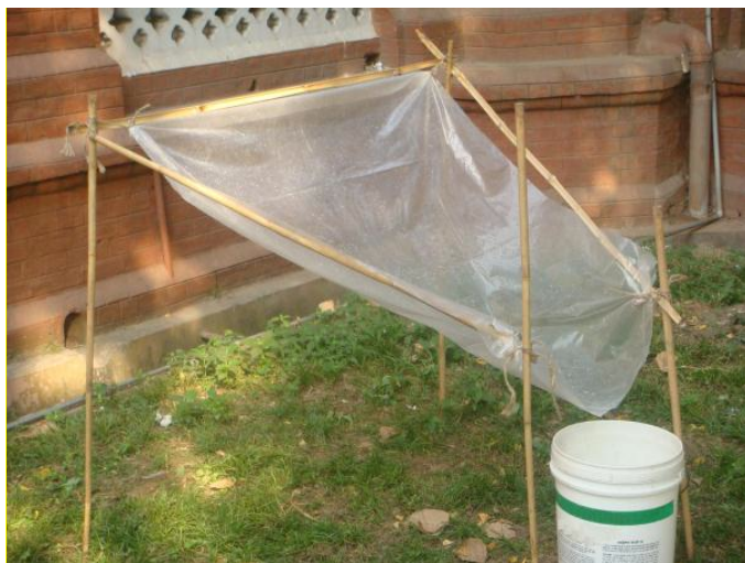
Figure 27 The construction of the rainwater collector with polyethene sheet, bamboo sticks and a bucket.
