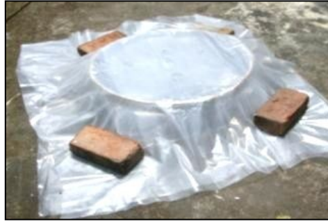
Figure 30 Place two polyethene sheets on top, as before and to create the two enclosed air layers on the top, place a few straws in between the sheets. Then expose it in the sun for about 1 ½ to 2 hours.
