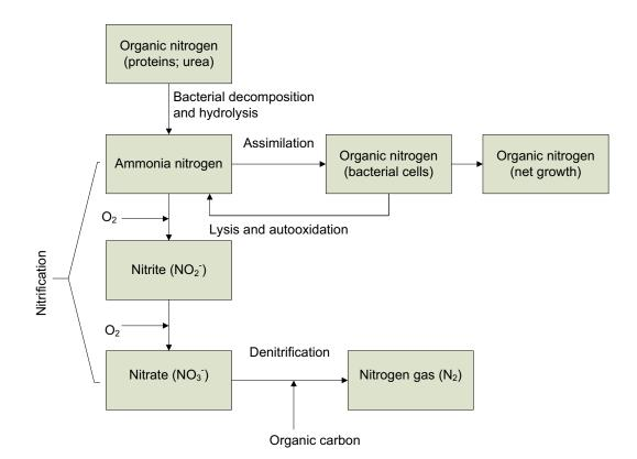
*Figure 4*. Nitrogen transformations in biological treatment (Tchobanoglous et al. 2003).
