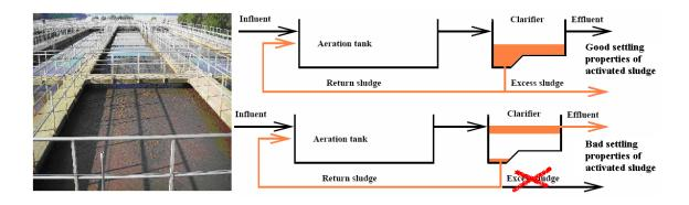
Figure 2. Bulking sludge in the clarifier, Himmerfjärden WWTP 2006.
