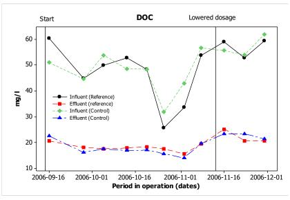
Figure 29 Influent and effluent DOC values for the control and experimental lines.
