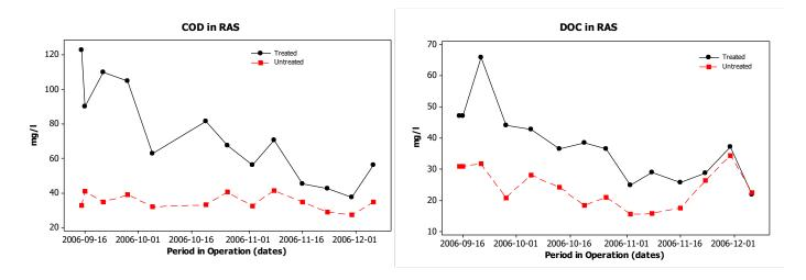
Figure 25. COD and DOC in the treated and untreated RAS in experimental line.
