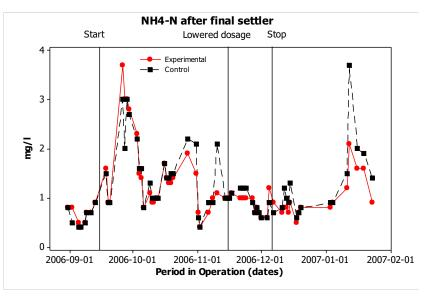
*Figure 30.* Ammonia in effluent of the tertiary treatment for the control and experimental line.
