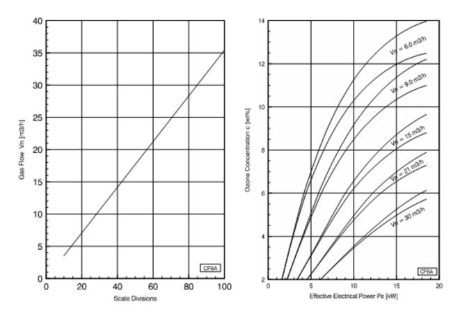
*Figure 8*. Gas flow and electrical effect diagram examples for the OZAT<sup>®</sup> OZONGENERATOR TYP CF-6A.
