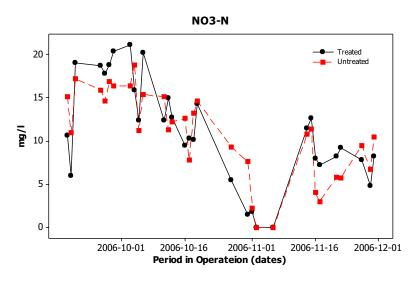
Figure 27. Nitrate (NO<sub>3</sub>-N) in the treated and untreated RAS in experimental line.
