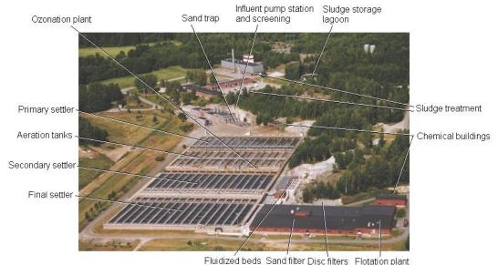
*Figure 9.* Overview of Himmerfjärden WWTP. The capacity of the biological and chemical unit is  $3.9 \text{ m}^3 \text{s}^{-1}$  and towards the mechanical unit  $5.2 \text{ m}^3 \text{s}^{-1}$ .
