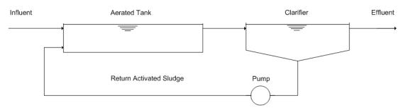
*Figure 1*. The activated sludge process, the waste water flow in to the aerated tank and out from the clarifier.
