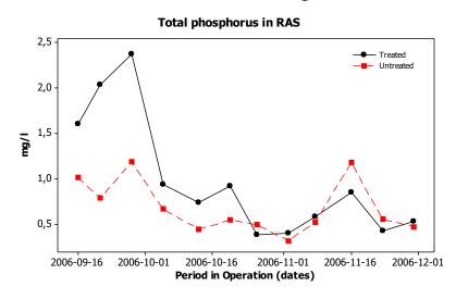
*Figure 26.* Total phosphorus (P-tot) in the treated and untreated RAS in experimental line.
