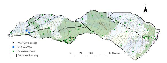
*Figure 5:* Studibach with the location of the seven nested sub-catchments and the 51 groundwater wells. Data Source for the background image: PK10; 1:10'000; (Federal Office of Topography Swisstopo, Bern))
