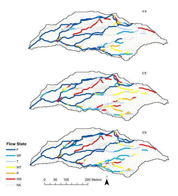
*Figure 41: Maps of the stream network from Campaign 4 to 6. With the mapped flow state according to the classification system.*
