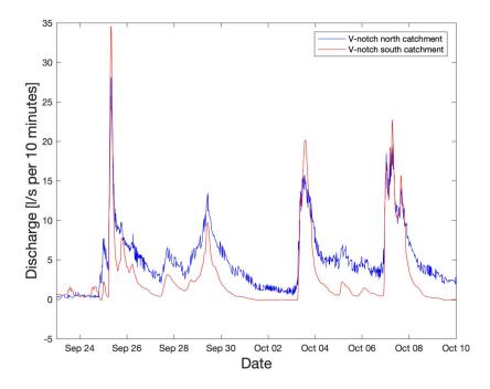
*Figure 56:* Discharge from the two different v-notches located below the south and the north part of the catchment.
