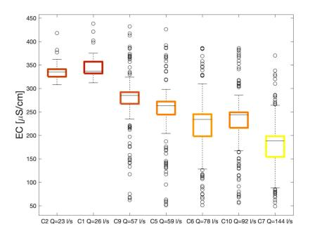
**Figure 24:** Boxplots of the EC for each measurement campaign sorted by the mean daily discharge during the campaign. The box represents the 25th-75th percentile, the line the median and the whiskers extend to the most extreme value not considered as outliers. The circles represent all outliers. The colors indicates the EC with red as high and yellow as low. Spearman's  $\rho$ =-0.64 and p=2.22e-114, correlating EC and Q.
