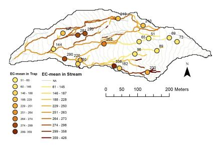
*Figure 27: Map displaying the mean EC of the water collected in the traps during campaigns C6, C7 and C9 (circles) and the mean EC of stream water during all seven EC-campaigns (lines).*
