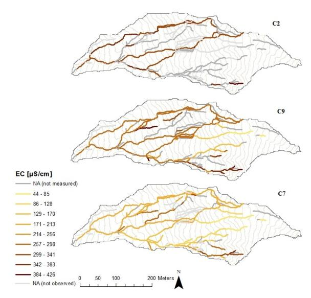
*Figure 20:* Maps of stream water EC in the lower Studibach catchment during three different field campaigns: C2, C7 and C9. In these campaigns the EC was highest during C2 and the lowest during C7, which had the highest discharge at the Studibach outlet, with 144 l/s. Discharge was 23 l/s during C2 and was 57 l/s during C9.
