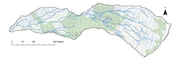
**Figure 4:** Studibach catchment and the stream network. There is only one stream that connects the upper part and the lower part. Notice that the stream network in the lower part is less dense than in the upper part. The streams in the upper part has previously been mapped, whereas the streams in lower part are derived from the DEM. Data Source for the background image: PK10; 1:10'000; (Federal Office of Topography Swisstopo, Bern)
