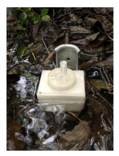
*Figure 11:* An EC-trap installed in a stream.
