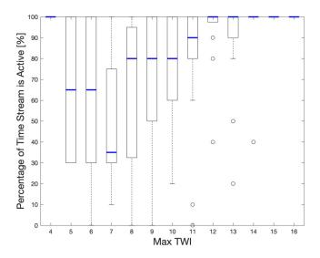
**Figure 48:** Boxplot showing the percentage of campaigns the streams were active related to the maximum TWI-values for each segment. Stream sections that were never active have 0 on the x-axis and stream sections that were always active will have 100 on the x-axis. TWI-values are rounded to integers.
