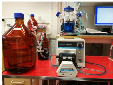
Figure 13: The setup for determining the RTD with methylene blue.
