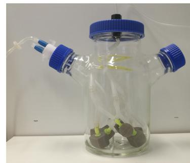
Figure 21: The adjusted aquarium air diffuser stone setup, with gas inlet at the top and a gas outlet with a back valve installed on the left side.
