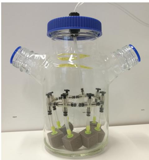
Figure 18: Aquarium air diffuser stones, connected to a tube supplying ozone-containing gas. NOTE: The setup is not in operative state.
