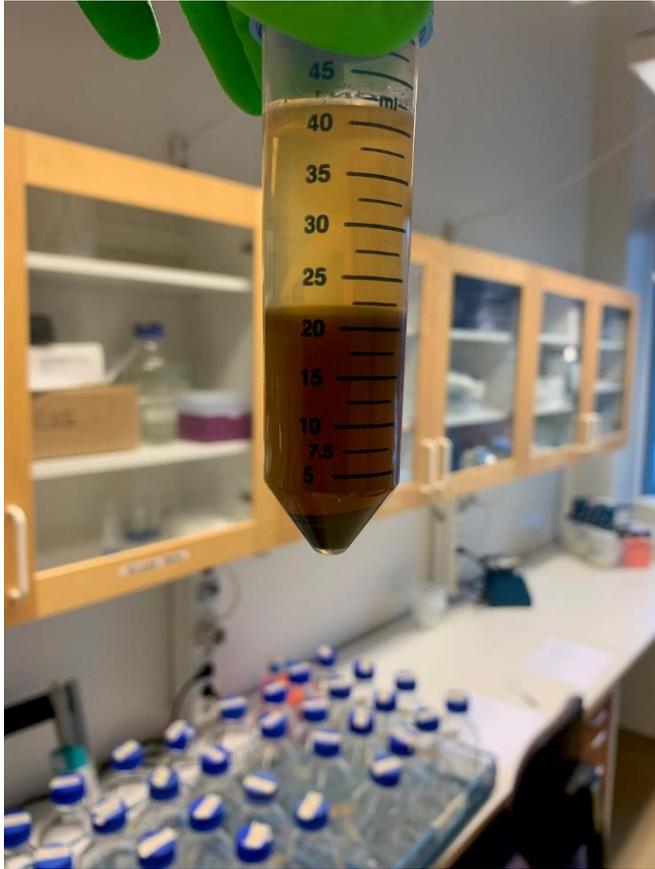
Figure 6. Nycodenz extraction process right after centrifugation. Compare to Fig. 5 - the soil slurry has passed through the nycodenz, and heavier particles can be seen at the bottom. On top of the brown soil-mixed nycodenz layer, just above the 20 ml mark, the thin grey-white layer of bacterial cells can be seen.
