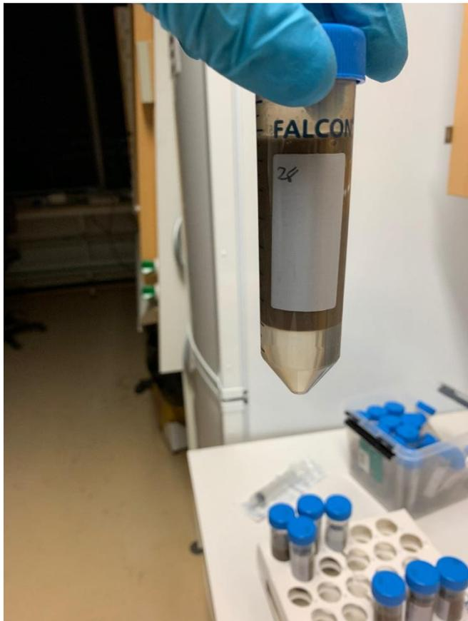
Figure 5. A 10 ml Nycodenz "cushion" has been added below 30 ml soil slurry in a Falcon tube. The next step was to centrifuge the tube.
