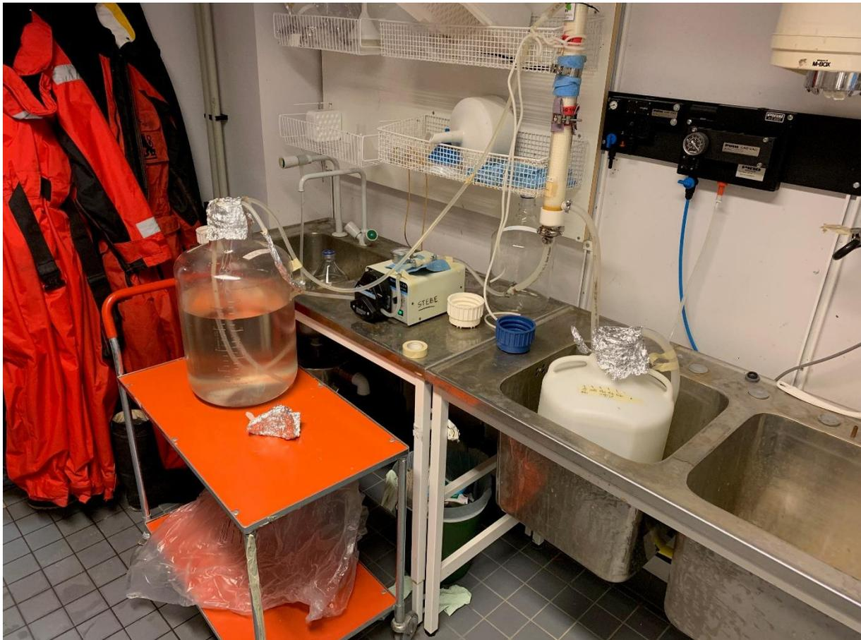
Figure 2. Setup of the tangential flow filtration (TFF) of the lake water for media and aquatic bacterial inoculum.
