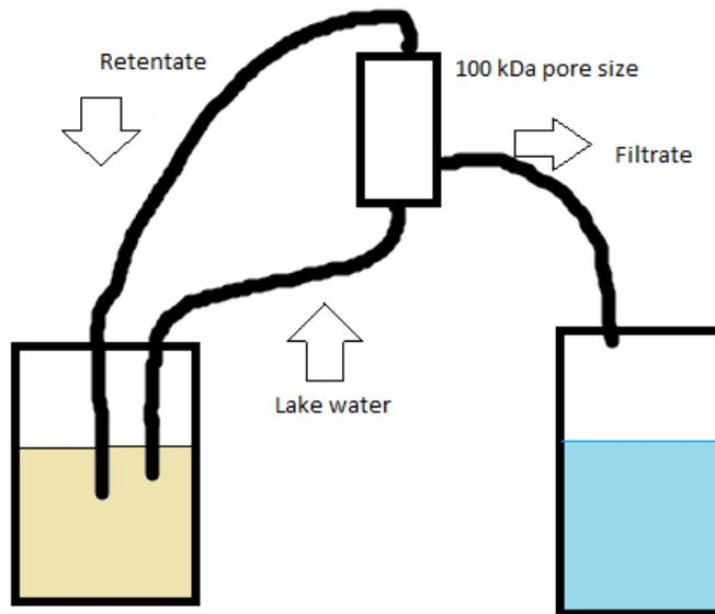
Figure 3. Depiction of the lake water filtration setup for media and Aquatic bacteria inoculum. The carboy to the left contained lake water. The carboy on the right was filled with sterile filtrate to be used as media in all bottles in the experiment. The retentate from the filtration was returned to the lake water carboy with the aim of concentrating lake bacteria there. This was then used as inoculum for aquatic communities.
