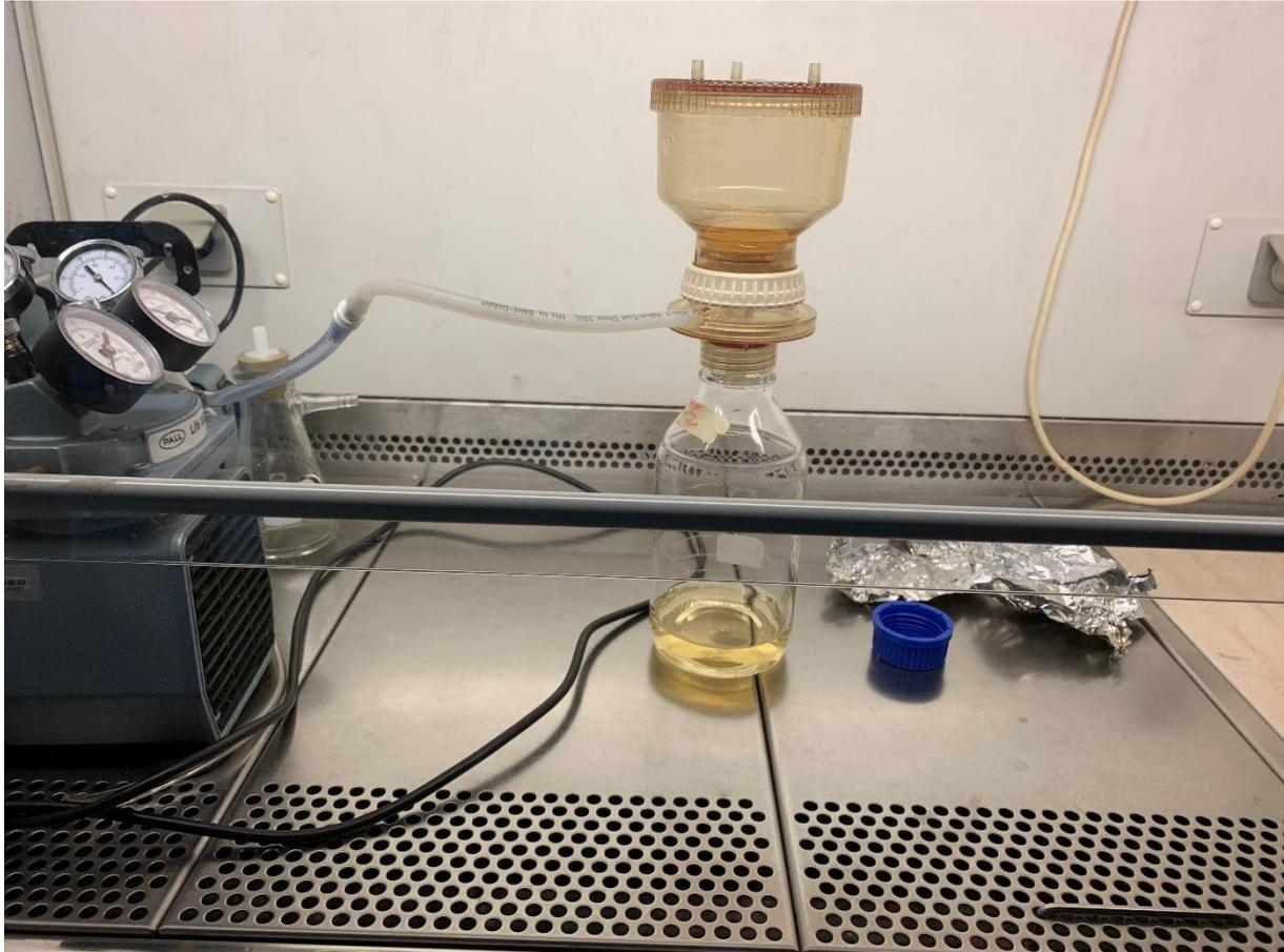
Figure 4. Sterile 0.1  $\mu\text{m}$  pore size filtration of soil DOM for “DOM” treatments, conducted in a laminar flow hood to maintain sterility.
