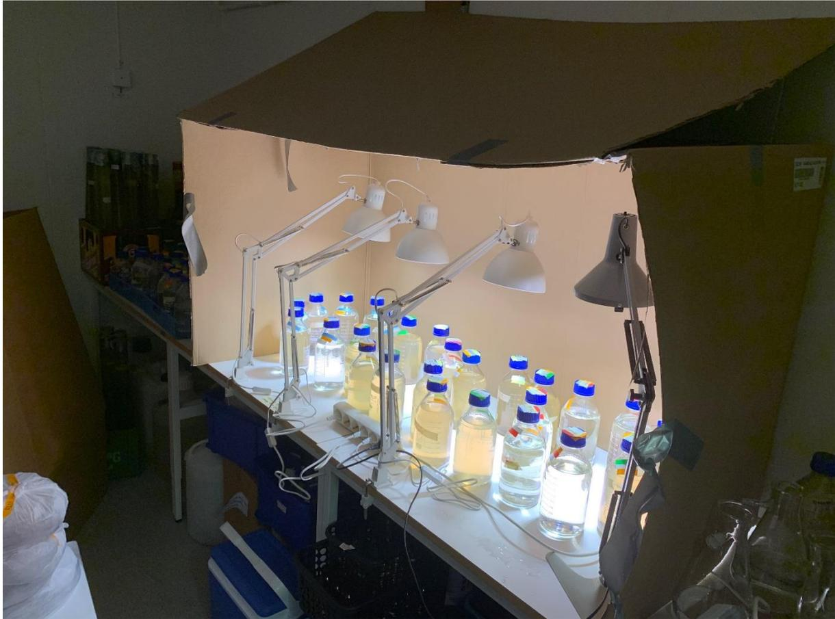
Figure 1. The experimental setup in the 4°C – room. Light treatments are scattered around the lamps; dark treatments are seen in the left of the picture. When the experiment was running, the cardboard box was closed to avoid light contamination.
