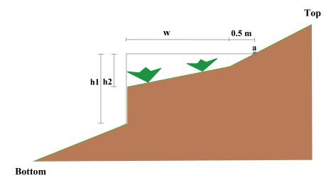
Figure 13. Illustration of the measurement setup to evaluate the terrace volume in the Example Landscape in Son La.
