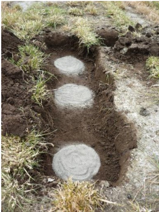
Figure 22: Set up before measurement with Disc permeameter is performed. Contact sand is placed on the ground in the shape of the disc.
