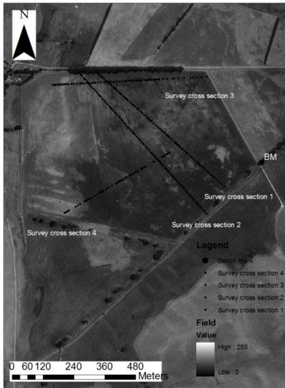
Figure 18: Cross sections for level survey.
