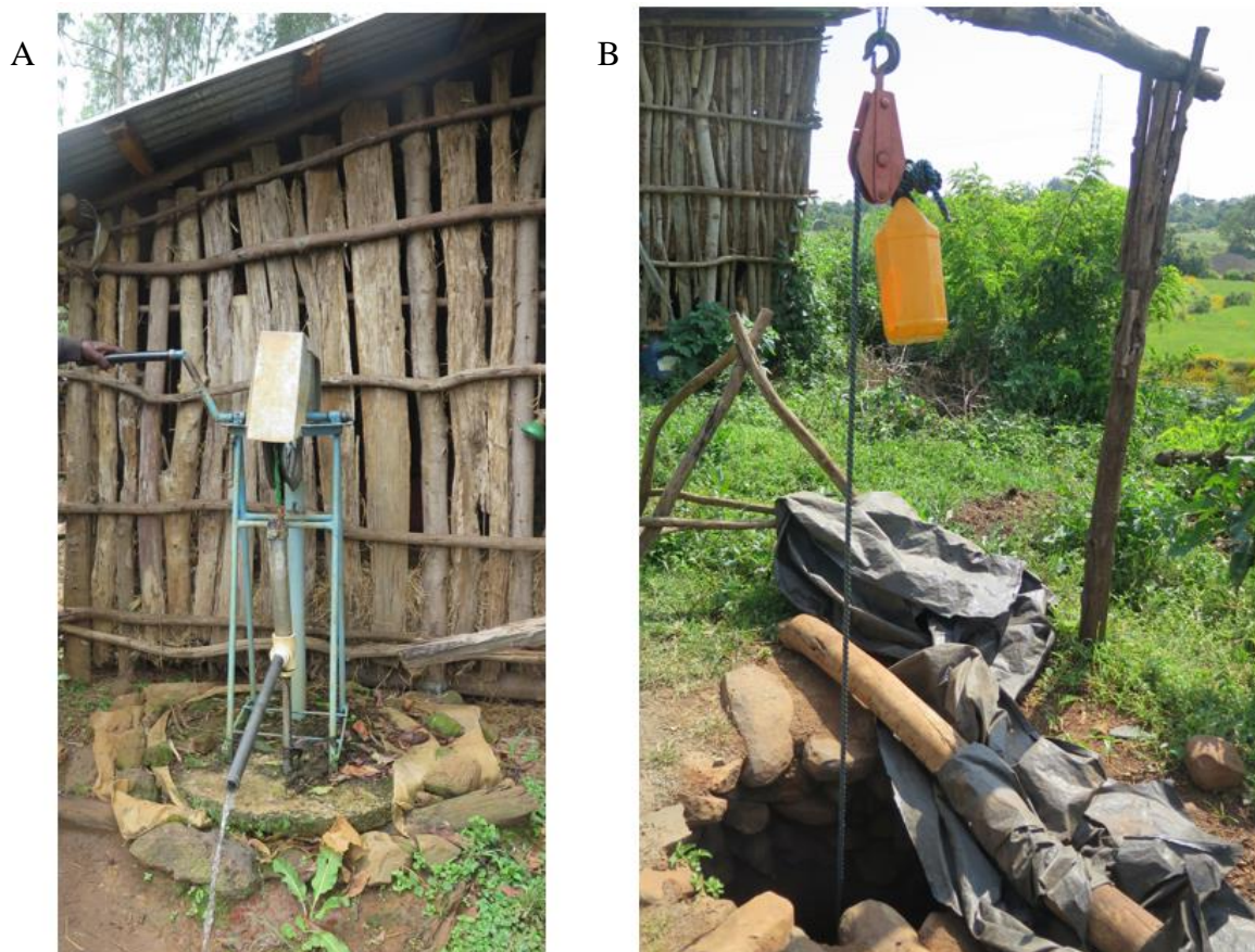
Figure 3. A) The rope and washer pump technique. B): The pulley and bucket water abstraction technique (Larsson, 2018).
