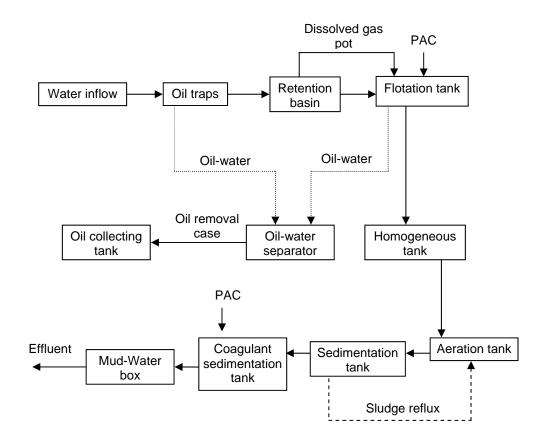
Figure 19: The coking plant wastewater treatment plant.
