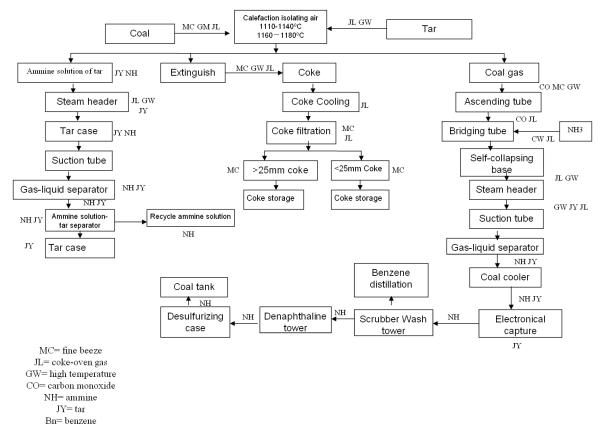
Figure 18: Process scheme from the coking plant.
