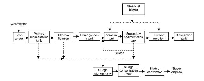
Figure 17: Paper mill oil wastewater treatment.
