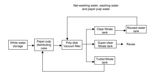
Figure 16: Paper mill recycling of water.
