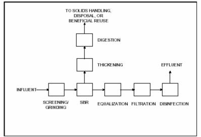
**Figure 2:** A typical process flow schematic for a municipal wastewater treatment plant using an SBR (Wastewater technology fact sheet, 1999).
