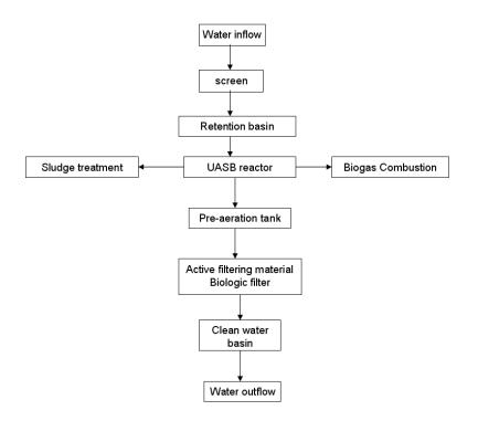
Figure 24: Wastewater treatment of Kernel Bio-Pesticide.
