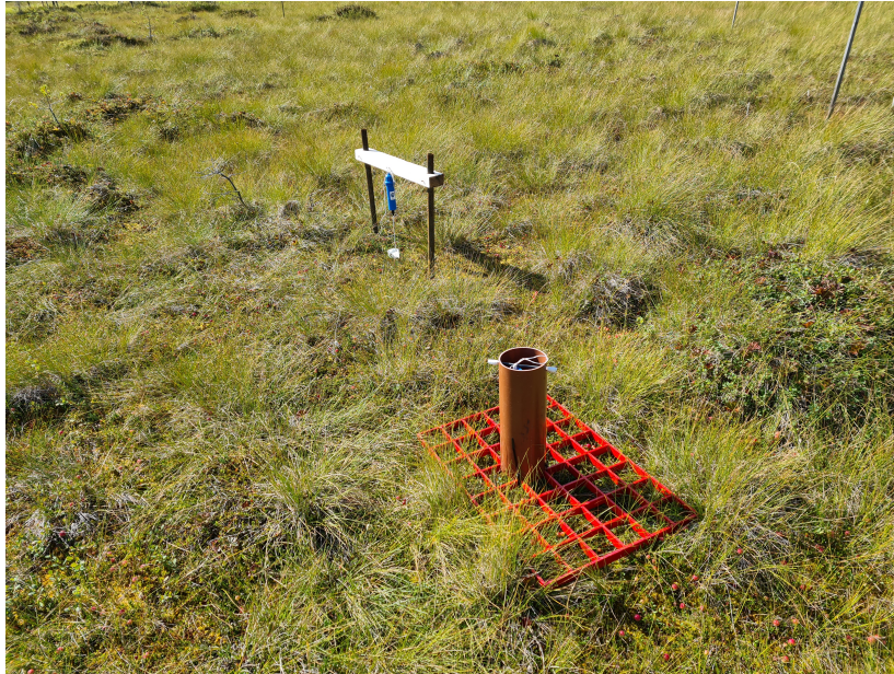
Figure 6: Photo of the groundwater level measurement setup with a pair of loggers at one of the mires on the chronosequence (site 29).
