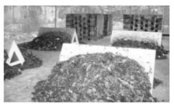
**Figure 3** Waste piled onto and around triangular aerators as it can look in Bangladesh (Rothenberger & Enayetullah, 2006).
