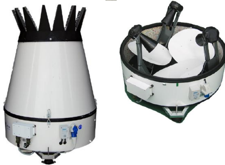
Figure 6. The trailer that contains the AQ 500 Wind Finder sodar system and the antenna unit with and without the wind shield (AQSystem, 2008).
