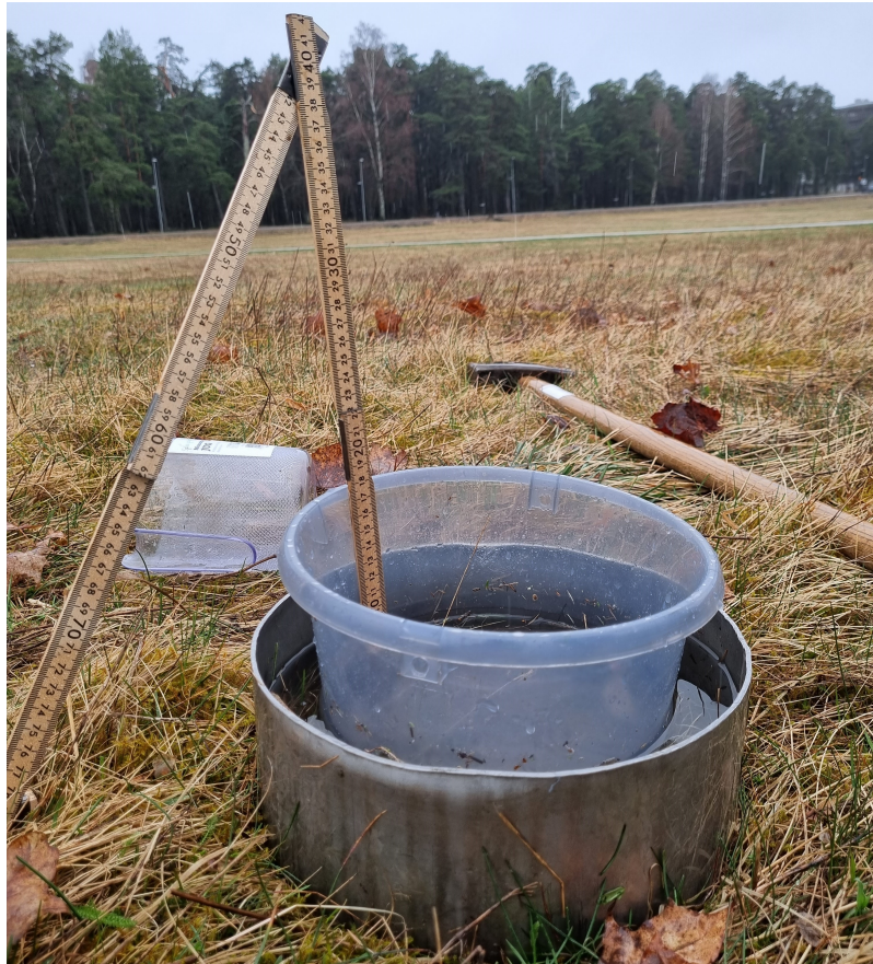
Figure 7: Infiltration measurements setup (Photo: Anastasia Novikova)
