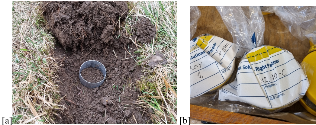
Figure 6: Soil sample collection using the core cutter method (a - b) for bulk density measurements in the lab (Photo: Anastasia Novikova)
