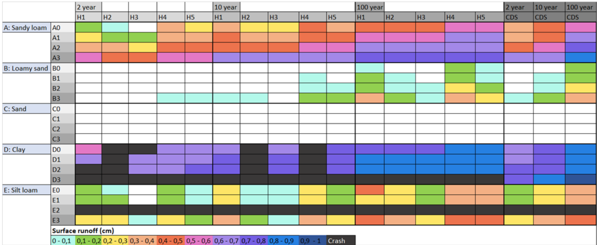
Figure 12: Runoff coefficient for each type of soil, degree of compaction, hyetograph and 2,10 and 100-year rain
