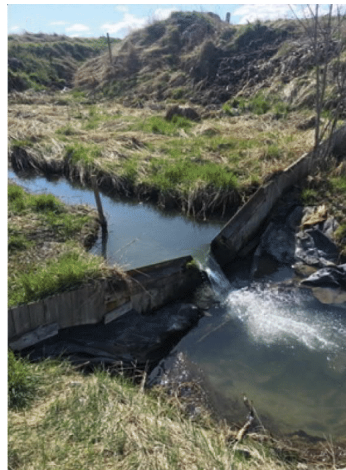
Figure 2: The measurement location in the Sundbromark-catchment in May 2018. The sensors, except the pressure transducer, is placed under water on the wooden rod just upstream the V- notch weir.
