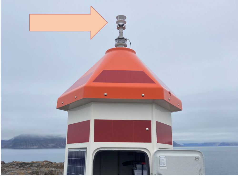
Figure 6: Setup of AWS on a pole, attached to the roof on a lighthouse. Arrow points at the AWS (MaxiMet GMX500).
